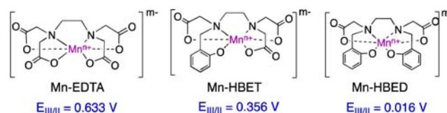
Figure 1. Ligand structure strongly influences the redox potential of the Mn III /Mn II couple. Conversion of carboxylato to phenolato donors shifts the half-cell potential by 617 mV in favor of the higher oxidation state.
